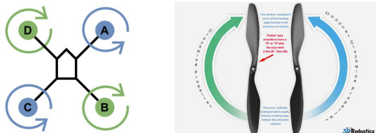
Figure 1: Propeller Configuration and Direction (Left) and Propeller Shape (Right)
